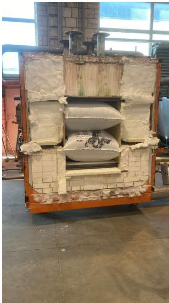
Module secured against collapsing lining
